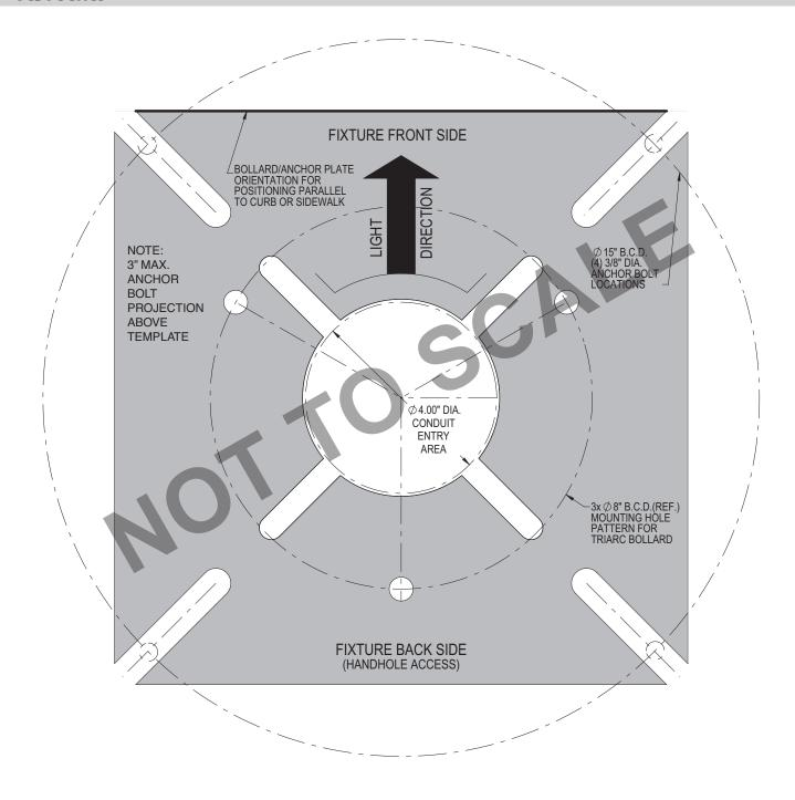
The sample template above is not to scale and is not intended for actual use on-site. Scaled template will be shipped with every pole or anchor bolt order.
