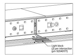
**B.** To prevent light leak, bend LED shield and install by snapping (4) outer tabs into (4) wireway mount slots at all fixture intersections.
