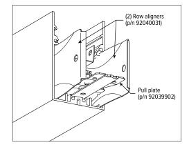
**B.** Remove (2) screws from parking holes and place in pull plate alignment holes to secure the pull plate to the newly placed fixture.
