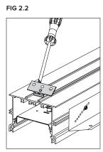
B. Reinstall access plate and use a flat blade screwdriver to pry hanger brackets upward 90° to provide access to the suspension holes. See FIG 2.2
