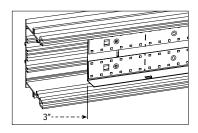
B. Slide fixtures together, engaging row aligners into joining fixture.
