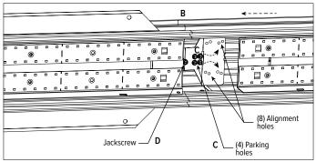
D. Using center located jackscrew, draw the 2 fixtures tightly together. Do not over tighten.
