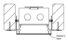
C. Attach ceiling material through the backer flanges and in to the support structure. See FIG 4.2
