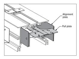
C. Remove (4) screws from parking holes and place in alignment holes to secure the row aligner to the newly placed fixture.
