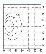
Footcandle calculations based on standard building reflectance of .10 with a ground reflectance of .0 and a light loss factor of .90.
